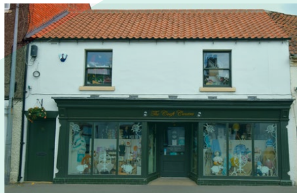
Where shopfronts extend across the majority of the building, the use of more substantial pilasters and facias, along with a dark colour act to visually support the upper floors.
